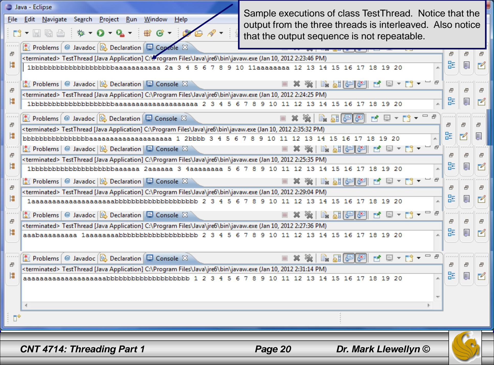
Sample executions of class TestThread. Notice that the output from the three threads is interleaved. Also notice that the output sequence is not repeatable.
