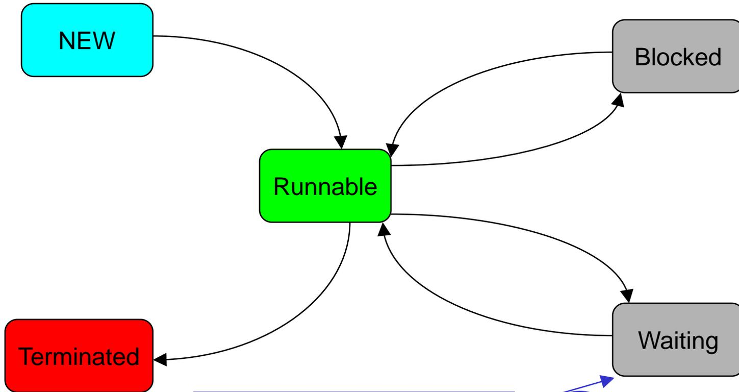
If the thread invokes the `wait()` method, it is put into the waiting state and will remain there until another thread invokes the `notify()` or `notifyAll()` method.
