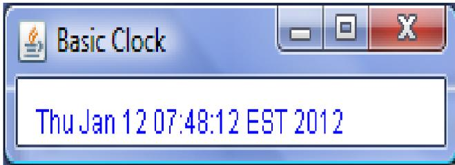
Date() returns current time to the millisecond. toString() method returns a textual representation of the date in the form: *w c d h:m:s z y*
